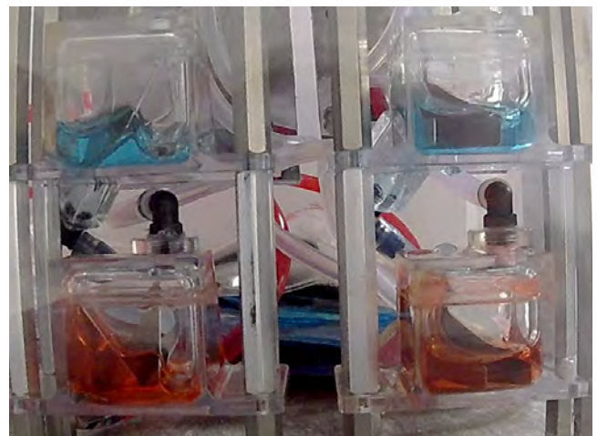
Figure 2. Low-fill fraction results for trapezoidal tanks, left column, and cube tanks, right column. Sloped face of the trapezoids faces away from the camera in this view. Drain of each tank is in the corner at the bottom, left, and into the page.
