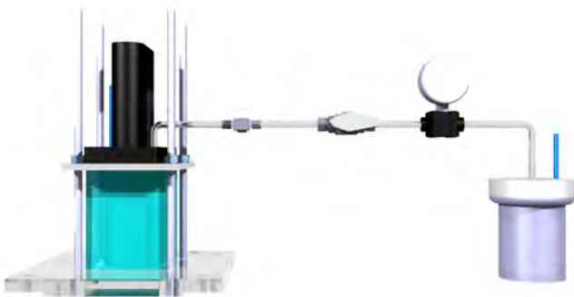
Figure 2: Experimental setup composed of quartz sloshing cell (clear blue), heating reservoir (grey and white), connecting pipeline (light grey) and vacuum and filling port (blue).
