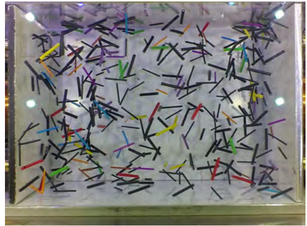
Figure 1: Granular gas mixture of rod-like particles with two different aspect ratios, image from the drop tower microgravity experiment (one of the views). The container dimensions are 11.2x8x8 cm.
