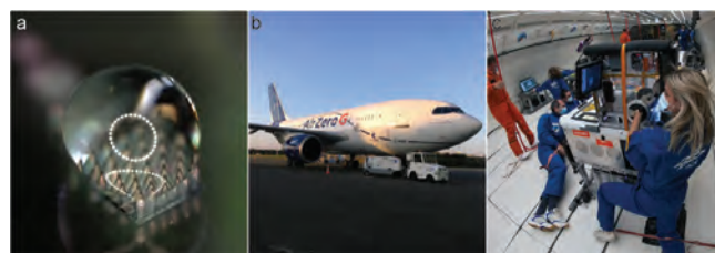
Figure 2: Experimentation on the NIMFS. (a) High surface tension, increased contact angle and water intake was noticeable during ground-based experiments and (b, c) an increase in liquid intake can be anticipated during microgravity experiments at the 35 th DLR Parabolic Flight Campaign.
