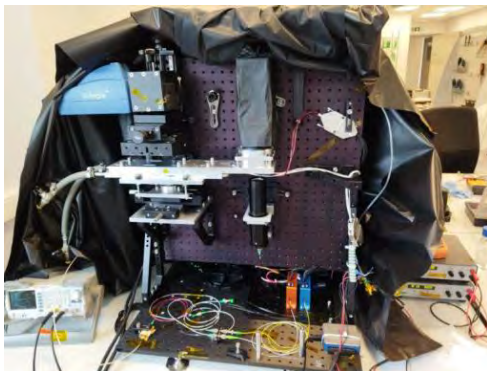
Figure 1: Picture of the bichromatic dynamic shadowgraph developed and validated during the phase C0.
