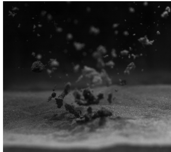
Figure 1: Ejecta Plume generated by impacting a basaltic projectile ( v = 65 \text{ cm/s} ) in a bed of 0\text{-}300 \mu\text{m} sized particles at a gravity level of 2 \cdot 10^{-4} \text{ m/s}^2
